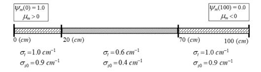
Figure 2: Heterogeneous benchmark problem used to compare the proposed ELD-SN method with DD, LN and SGF methods.
