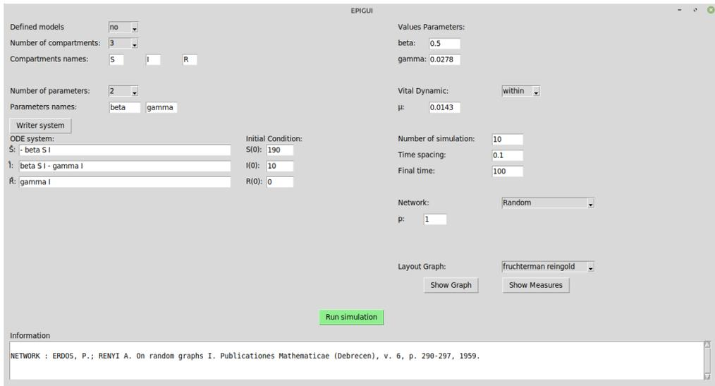
Figure 2: The EPIGUI interface. In this interface, the user is able to set up the number of compartments, parameters and write the correspondent equation. Additionally, the type of network and respective parameters are also disposable to be configured.
