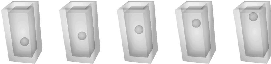
Figure 4: Single bubble rising in a continuous phase, for  $t = 0.015 \text{ s}$ ,  $t = 0.030 \text{ s}$ ,  $t = 0.045 \text{ s}$ ,  $t = 0.06 \text{ s}$  and  $t = 0.075 \text{ s}$ . Here,  $Re = 30$  and  $Eo = 2$ .
